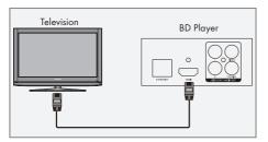
1 Connect the HDMI cable enclosed into the »HDMI« socket on the back of the device and the corresponding socket (HDMI) on the LED/ LCD TV.
